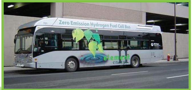
Hydrogen fuel cell bus. Source: National Renewable Energy Laboratory (NREL) Photographic Information eXchange (PIX)# 16143
