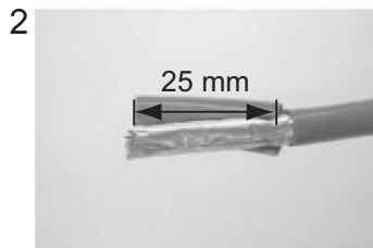
2 Remove the inner vinyl sheath by approx. 25 mm. Be careful not to damage inner shield and cores.
