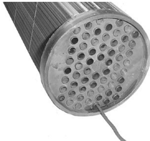
Clean Aftercooler Core
