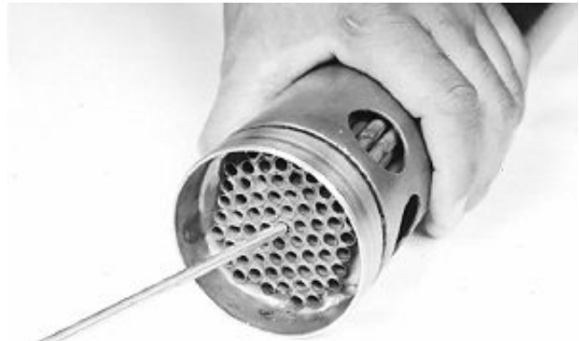
Clean Heat Exchanger
