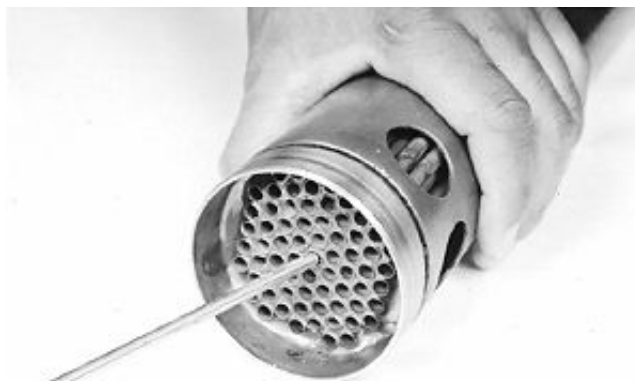
Clean Heat Exchanger
