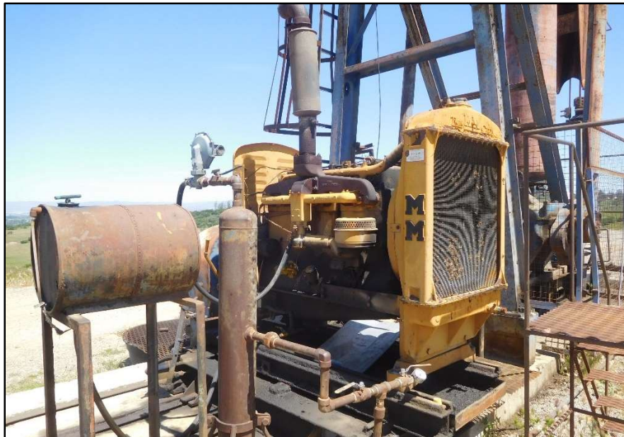
Figure 1.1 – Reciprocating Internal Combustion Engine
